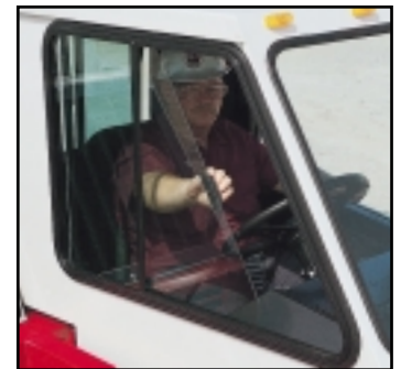
Right sliding window in carrier cab provides improved ventilation.
