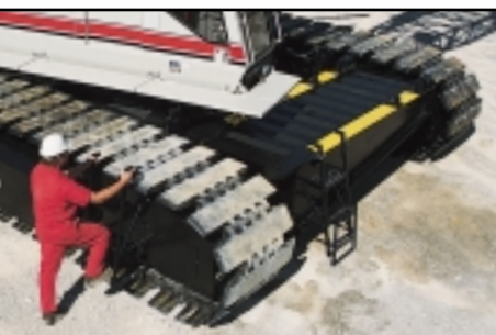
Counterweight tray, repositionable ladders and removal catwalks provide outstanding accessibility.
