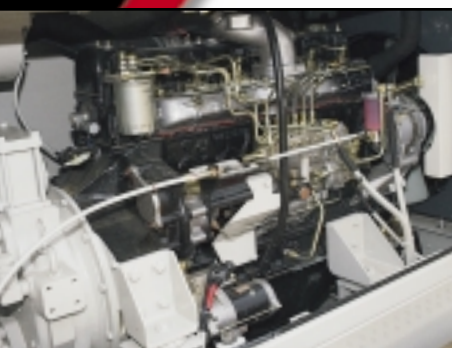
207 hp Isuzu A-6SD1T-QB engine
