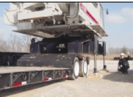
Hydraulic jacking system lifts the upper, lower frame and treadmembers off the ground. Treadmembers are removed and a trailer can then be backed under the lower frame and upper for transport.
