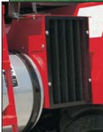
Transmission oil is cooled by a thermostatically-controlled oil cooler to provide maximum cooling under the most extreme job conditions.
