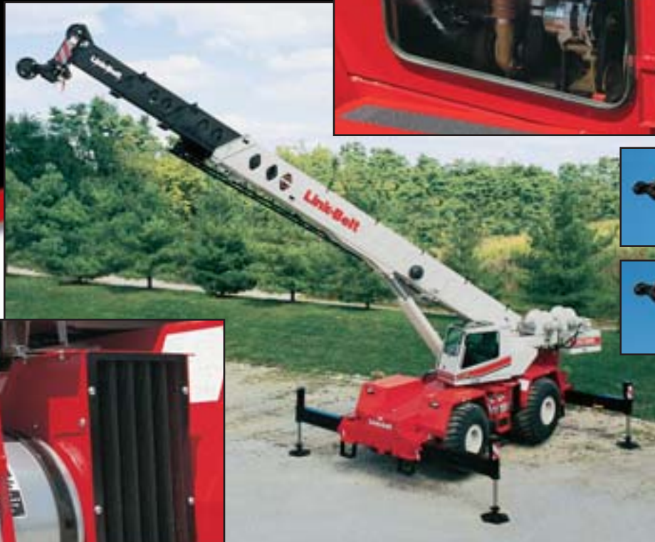
Transmission oil is cooled by a thermostatically-controlled oil cooler to provide maximum cooling under the most extreme job conditions.
