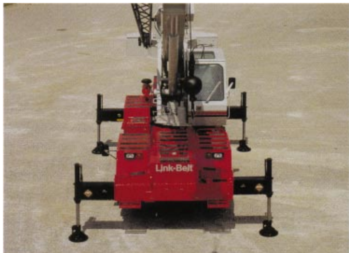
Intermediate Extended Outriggers – 12' 11-3/4" (3.96 m) spread
