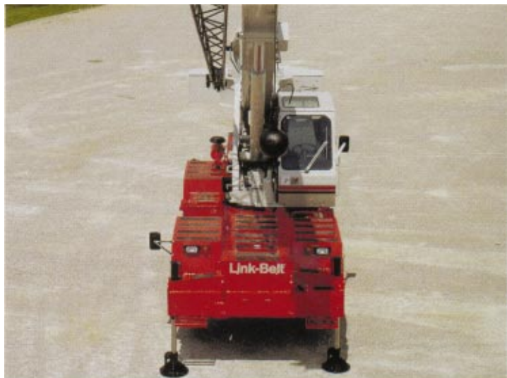
Fully Retracted Outriggers – 7' 4-3/4" (2.25 m) spread
